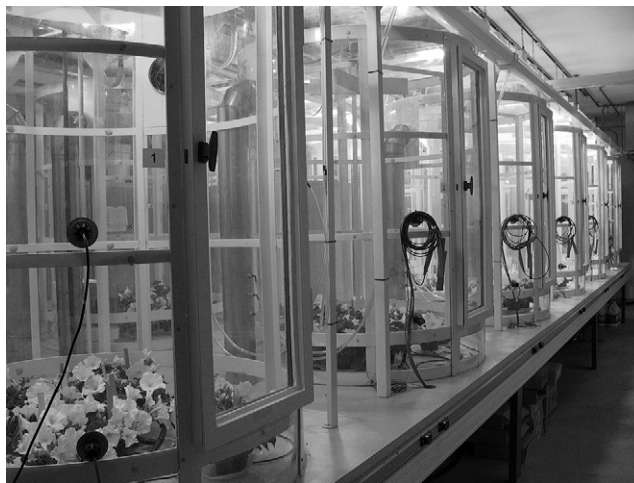
Fig. 1. Six of the 12 cylindrical chambers in which petunias were grown. The chambers have a 1:1 ratio (low light) or 2:1 ratio (high light) of HPS and MH lamps, a paddle fan mounted inside and at the top of each chamber to mix the air within the chambers, two thermocouples in each chamber to monitor temperature, and a humidity probe. CO 2 was added to half the chambers by a CO 2 controller. HPS = high-pressure sodium; MH = metal halide.
